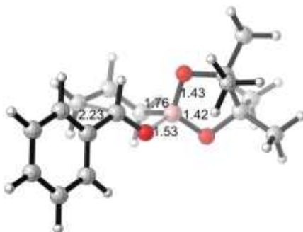
Figure 3.8 Optimized transition state of the uncatalyzed allylboration of benzaldehyde at the B3LYP/6-31G* level of theory.
